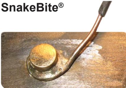
SnakeBite® - Patented PinBrazing connection for connecting anode leads without cable lugs. Just bend the wire to a round shape with the enclosed special plier and pinbrazed directly to the pipe.
