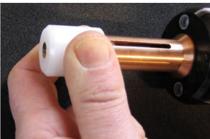
4. The lift level is calibrated when the brass rod is in same level as the outer plastic sleeve.
