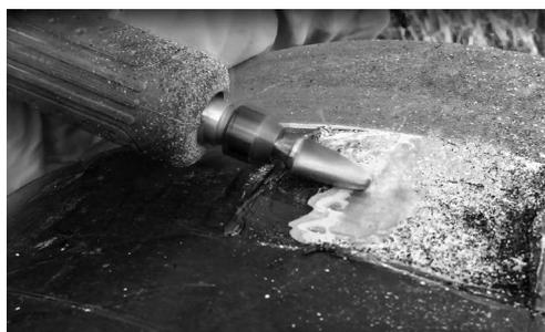
1. Grind the brazing and ground area until you have an even and clean surface.
