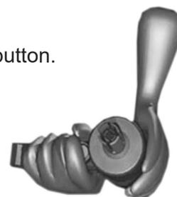
8. Hold the gun in place for 3-4 sec after the brazing while the brazing cools down.
